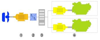
Figure 1: Setup of a diesel-electric drive train
