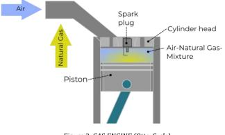
Figure 2: GAS ENGINE (Otto-Cycle)
