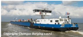
(gross) sufficient for the roundtrip Rotterdam - Basel ak IMO type C 20 % Vessel type: LNG-fuelled type G tanker ENI: 02324789 Vessel size: 110 × 11.40 m (L × W), Draught (max): 3.15 m Propulsion: Single 8L20DF Wärtsilä
