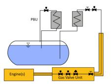
Figure 6: Pressure-build-up system (PBU)
