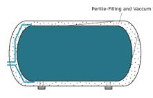
Figure 3: Pressure tank - vacuum insulated
