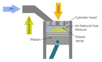
Figure 1: DUAL FUEL ENGINE (Diesel-cycle)
