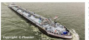
Vessel type: LNG-fuelled type C tanker ENI: 02337327 Vessel size: 110 × 11.4 m (L × W), Draught (max): 3.21 m Propulsion: Wärtsilä 6L20 DF dual fuel engine , 1100 kW Bunker capacity (LNG): 60 m<sup>3</sup> LNG tank: Wärtsilä LNGPac
